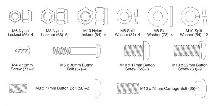
1. Attach one of the Stabilizers (19) to the front of the Frame (1) with two M10 x 75mm Carriage Bolts (65) and two M10 Nylon Locknuts (64).
